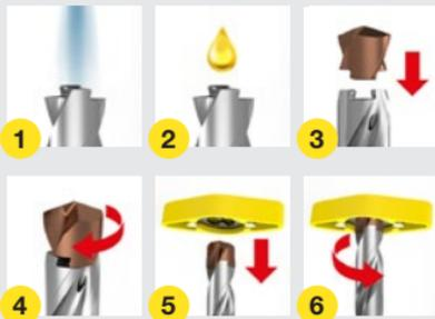
1. Clean the interface with air blast.
