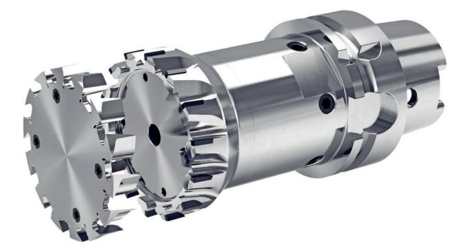
Thanks to its extraordinary technical details, Gühring's SMART CAP PCD face milling cutter makes it possible to achieve top productivity and energy efficiency in machining aluminium. The Smart Cap solution is produced by means of additive manufacturing and facilitates defined chip evacuation for maximum process reliability, an optimised supply of coolant and appropriate wear protection for the body.
