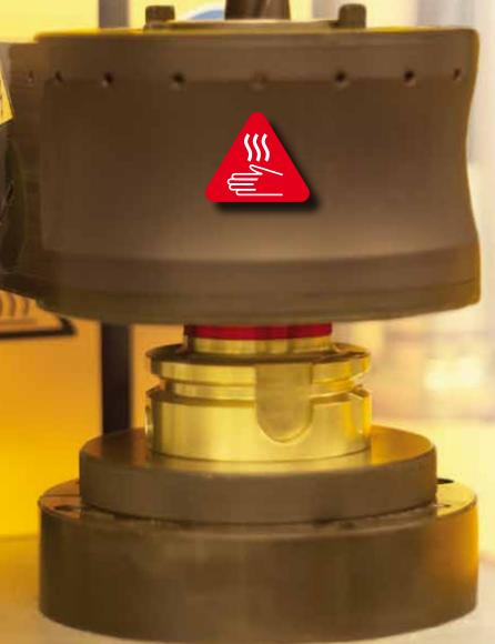
4. Blue ring: The cooling procedure is completed. The chuck now has a temperature below appr. 45° C.
