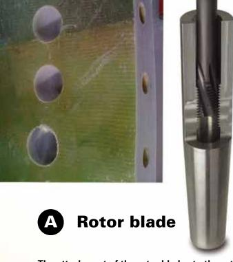
The attachment of the rotor blades to the rotor hub is one of the highly stressed areas of wind power stations. It requires accurate holes and load-bearing threads for the rotor blade and mounting bolts.
