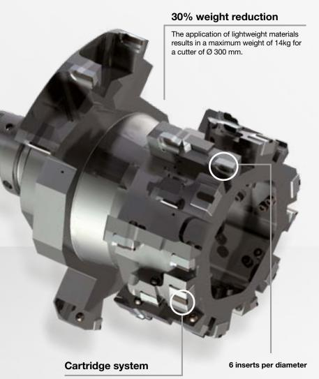
Thanks to exchangeable cartridges with PCD inserts and guide pads re-tipping the tool is quick and cost-efficient.
